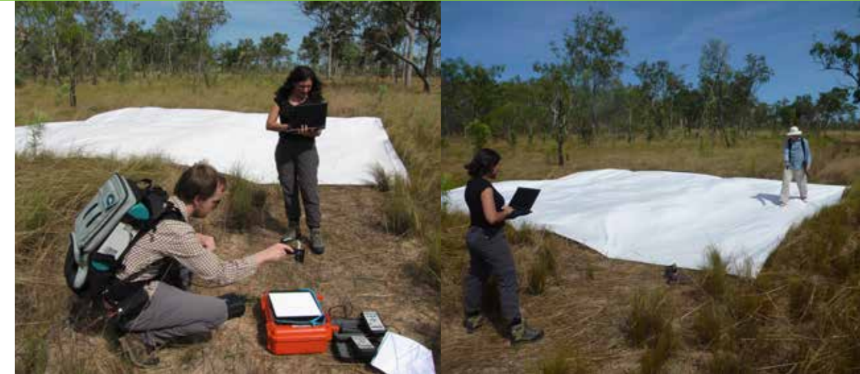
Above: (left to right) Field spectrometer calibration, validating calibration target for airborne data capture.
